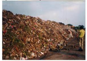
Figure 4.3 Bioculture is sprayed on the windrows.
