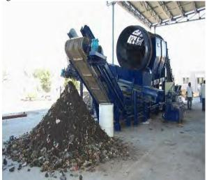
Figure 4.2 Segregation unit for separation of the organic and inert components.
